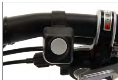
Button for pushing assistance
