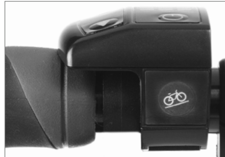
Button for pushing assistance
