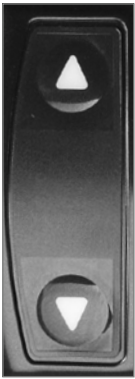
Buttons for power-assist level
