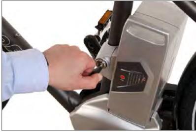
Unlocking the battery
