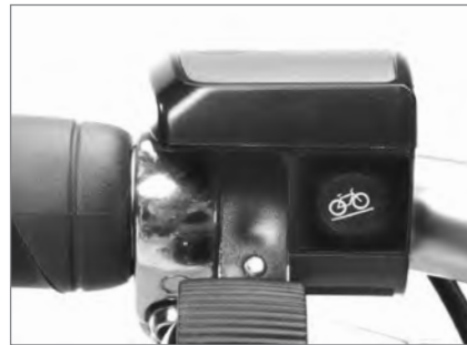
Button for pushing assistance
