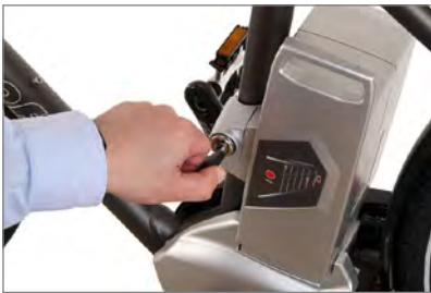
Unlocking the battery
