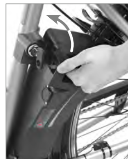
Reinstalling the battery
