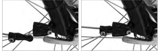
Safety mechanism released Safety mechanism engaged
