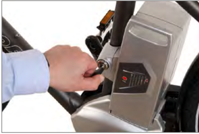
Unlocking the battery
