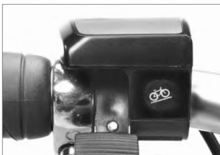
Button for pushing assistance
