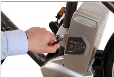
Unlocking the battery
