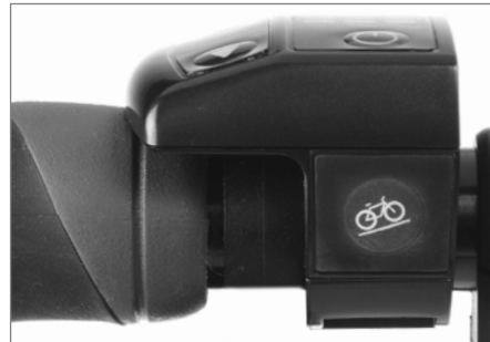
Button for pushing assistance
