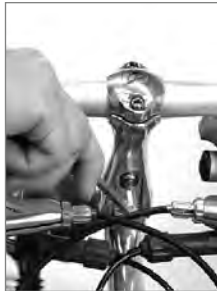
Hexagon socket screw (integrated stop notch)
