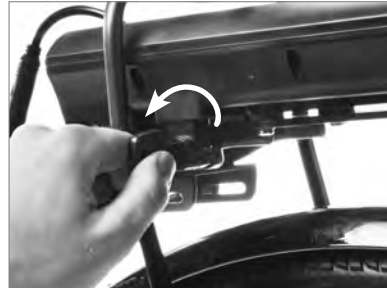
Unlocking the battery
