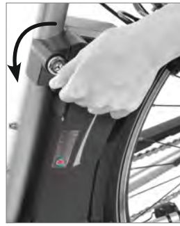
Unlocking the battery
