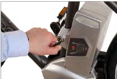
Unlocking the battery
