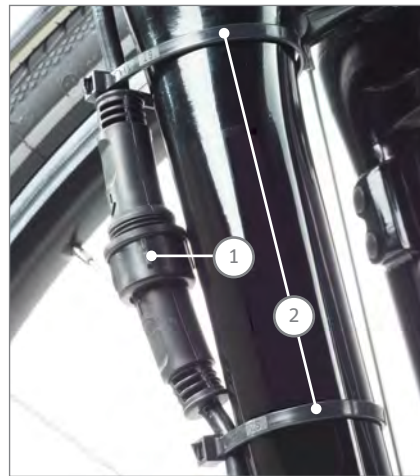
1 Locking nut 2 Cable tie
