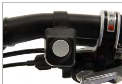
Button for pushing assistance
