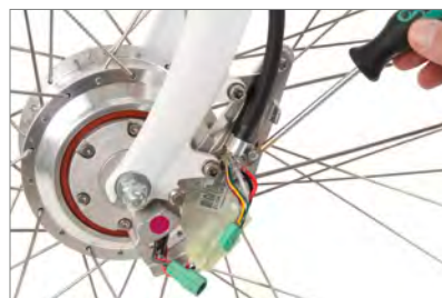
Base plate with cables and connectors
