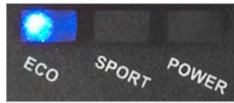
Display of power-assist mode
